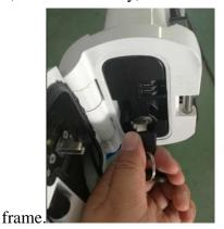
5, Hold the handle with your hand and pull out the battery
