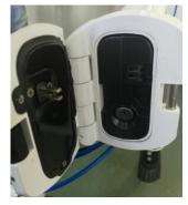
4,Insert the key, Turn the lock counterclockwise to unlock the battery and the
